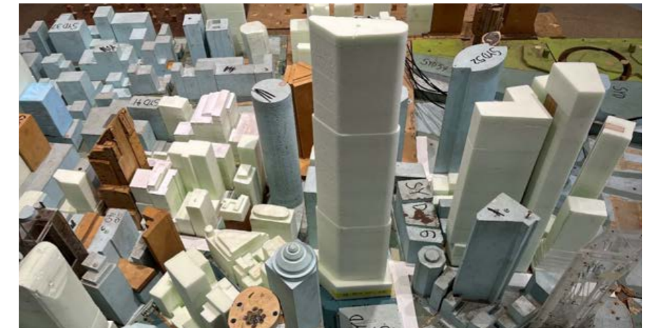
View from the East of base case - wind tunnel
